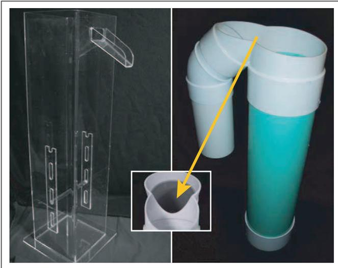
**Fig 1.** The standard model volumeter (Sammons Preston; Bollingbrook, IL) is on the left and our home use volumeter is on the right. Our volumeter is more precise because of the junction between the water cylinder and the spout (magnified view); it is lighter and easier to handle because it requires less water (10.6 v 22.5 L).
