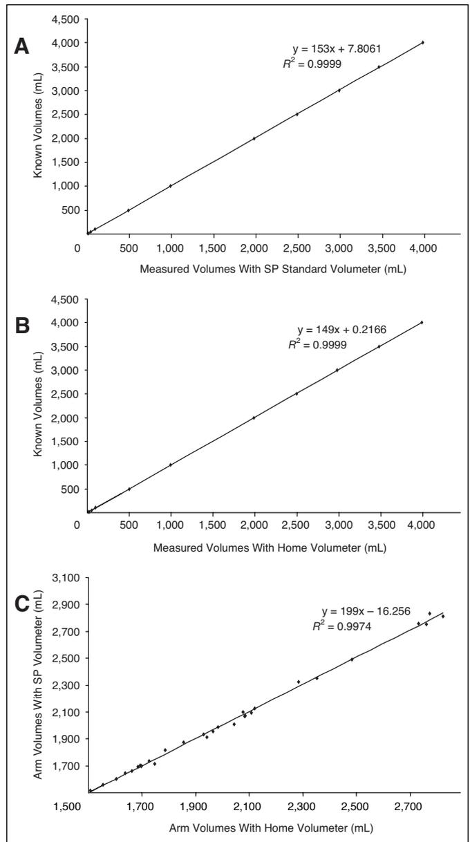
**Fig 2.** Scatterplots of the standard known volumes and the average measured volumes for each volumeter separately for the cast cylinders [(A) for the standard model volumeter; (B) for our home use volumeter], and (C) of the mean arm measurements with both volumeters. SP, Sammons Preston volumeter (Bollingbrook, IL).
