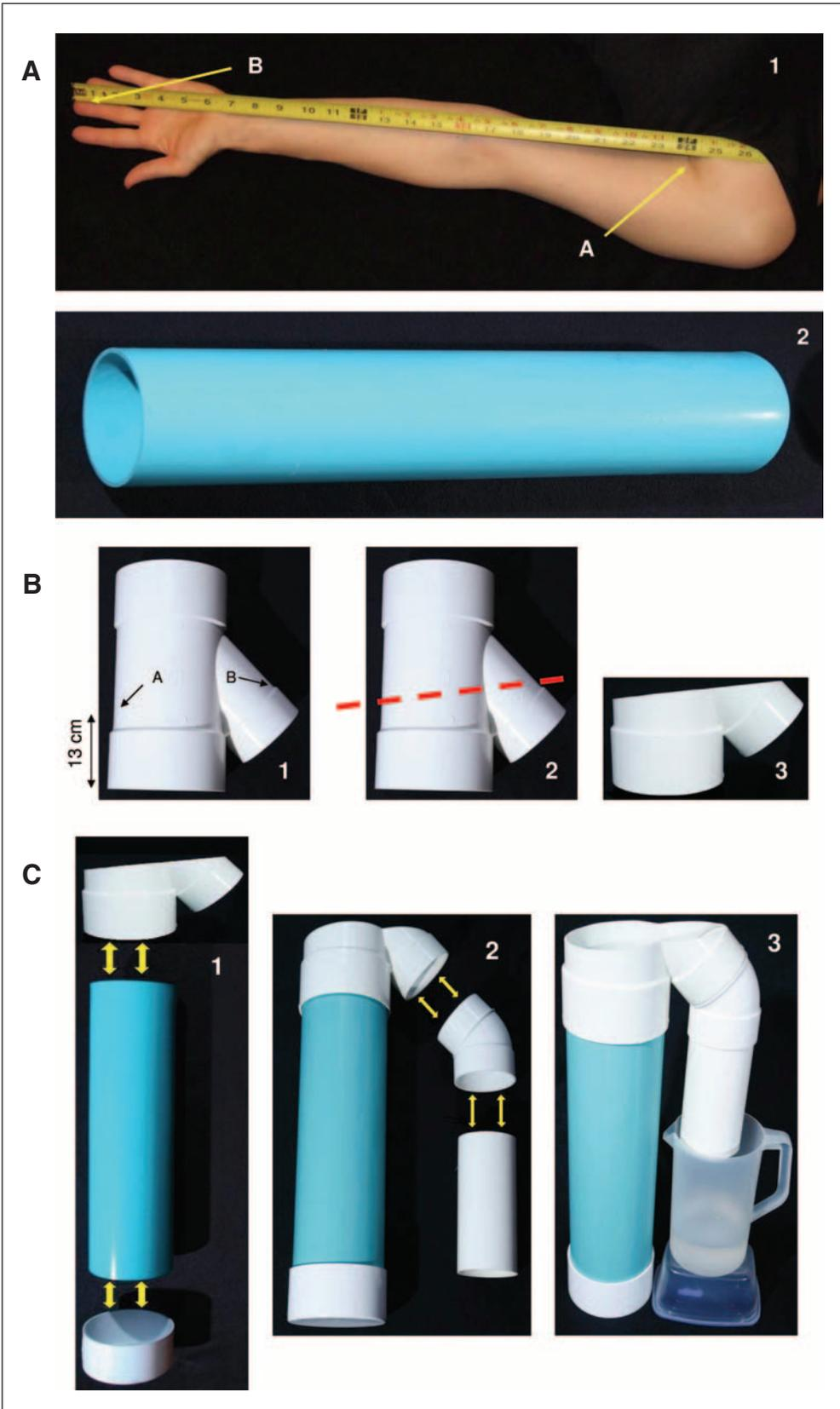
**Fig 3.** How to construct and use a home arm volumeter. (A, B) Preparation of parts, (C) assembly, and (D) arm volume measurement procedure, including a longitudinal cross-section view. (Continued on following page)
